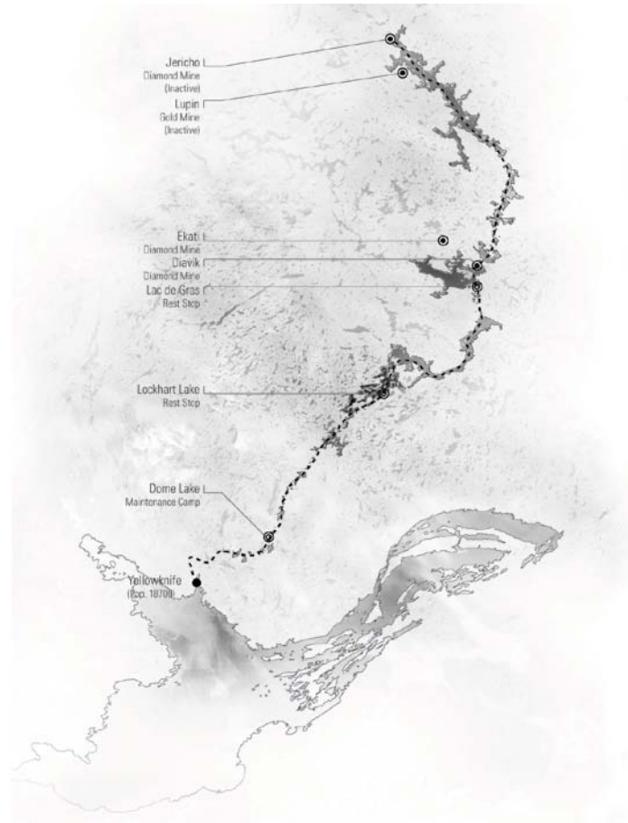
Fig 6. The Contwoyto Winter Road: First constructed in 1982 to offer access to remote mining sites, the road is almost 600km long with about 87% of its surface built on frozen lakes.
