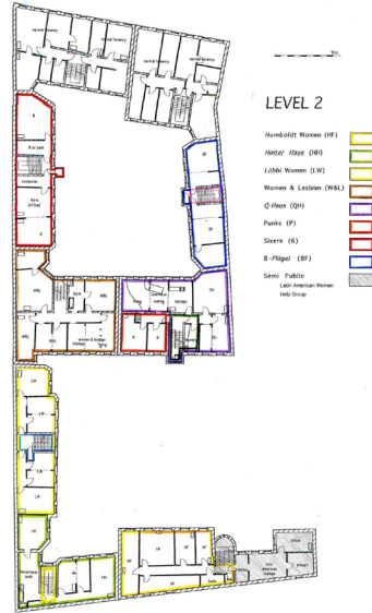
Fig. 15. The scale of various building sections influences group sizes and spaces. This means that the scale of occupancy is larger than single units, in many cases operating at the scale of an entire section of building. The Berlin courtyard building type is compatible with a complex and changing form of building occupation. The density of its arrangement, the even distribution of stairs wells, and its courtyard arrangement has a decisive influence on how the building is occupied. Images: Dougal Sheridan, 1994-1996.
