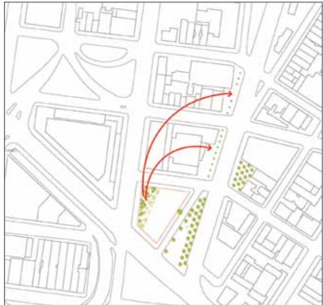
Fig. 24. In Year Three, after those trees reach a sufficient size they will be transferred to pits on neighboring streets to become street trees.
